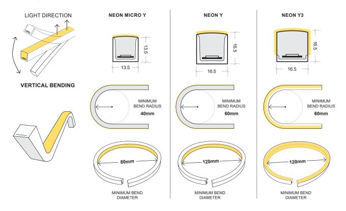
Exceeding these minimum bends may damage the product and cause segments to fail.
